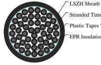
LSZH Sheath Stranded Tinned Copper Conductor Plastic Tapes Wrapping EPR Insulation
